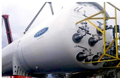
FILE: TANKS - Liquefied hydrogen has a temperature of -253 °C and is one of the coldest cryogenic gases there is, which places system components and materials under extreme strains. Once liquefied, hydrogen is reduced to 1/800th of its volume compared to that of its gas phase, facilitating a more-efficient distribution. But it needs fuel tanks four times the size of those for petrol.
